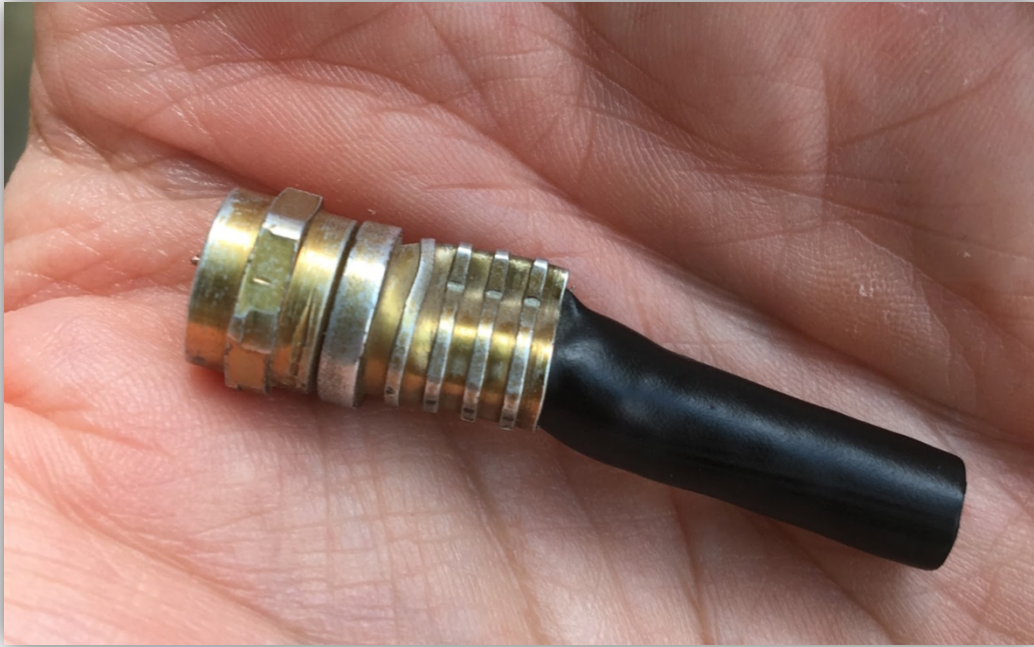
Figure 20: Crimp-on F-connector On Back of Modem Causing Micro-Reflection
