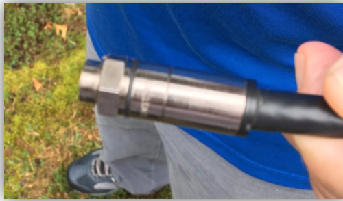
Figure 34: Bad Compression Type F-Connector
