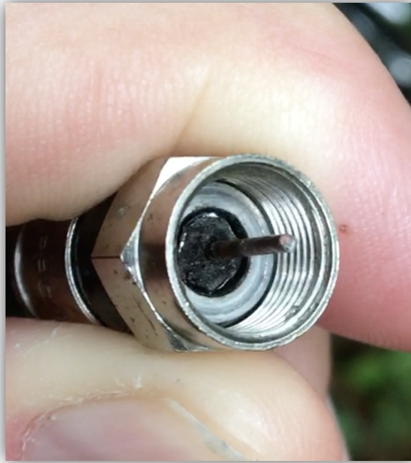
Figure 23: Blackening of Center Conductor and Insulating Dielectric Indicating Possible Surge
